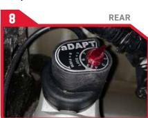
Adjust the "firm" setting on the shock
