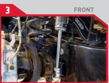
With the shock fully extended, rotate the shock shaft 360° in the direction of your desired setting.
