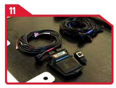
· Install the e-Adjust control module, wire harness and switch following the supplamental instructions.
