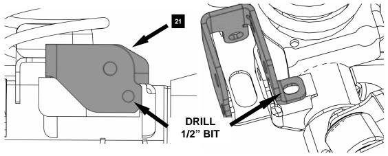
INSTALL ONE OF THE M12 BOLTS AND THE PROVIDED SERRATED NUT THROUGH
