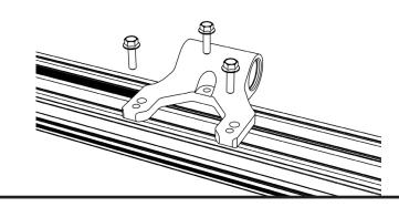
The Unita Cross Bars come with extra T-nuts that can be used to attach the bike mount, but M6 x 1.0 x 20mm bolts will be needed to attach the bike mount to the T-nuts.
