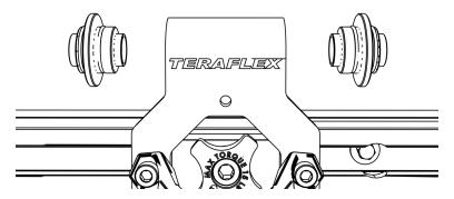
The spacers can be installed in either direction to fit 100mm - 110 mm.
