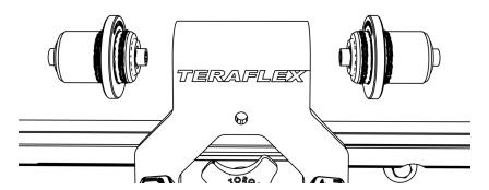
The spacers can be installed in either direction to fit 100mm - 135mm.
