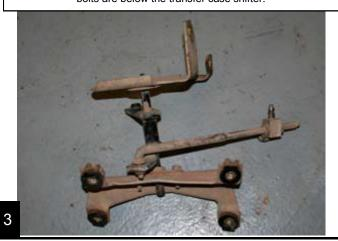
Install the new bracket onto the transfer case. Use the new flange nuts provided in the kit.
