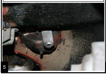
Assemble the shift linkage to the factory lever using the metal bushing to replace the plastic bushing in the lever. Note: We recommend using a thread locker on shift linkage fasteners.
