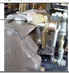
Remove the plastic bushing from the shift lever that sticks down through the floor of the body tub.
