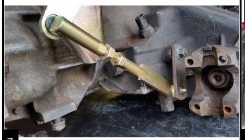
Adjust the length of the links and tighten the jam nuts. Some applications will require shortening of the upper threaded rod. Use caution when trimming to ensure that too much is not removed. We recommend using the "neutral" position as a starting point.
