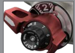
ADJUSTABLE COMPRESSION DAMPING
