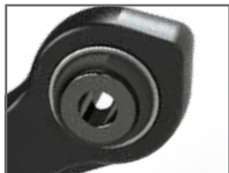
RUBBER BUSHING FOR REDUCED NVH
