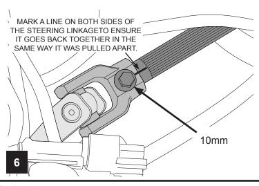
THE STEERING LINKAGE WILL NEED TO BE DISCONNECTED TO REMOVE THE DRIVER SIDE UPPER CONTROL ARM.
