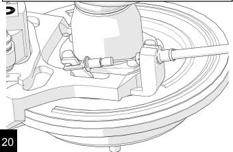
Reinstall tires torqueing lug nuts to 110 ft-lbs. Set the vehicle on the ground. Attach the emergency brake cables to the bracket under the body.
