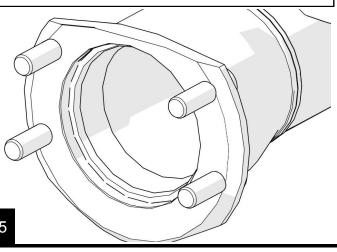
For semi-float applications— Press the old bearings and seals from the axle shafts. Do NOT remove bearings and seals for c-clip axles.
