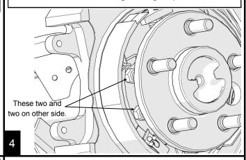
Remove the backing plate and wipe the bearing pocket surface clean of grease and contaminants.
