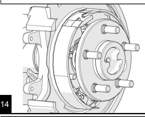
Install and tighten the nuts onto the retainer bolts through the access holes in the axle shaft with a 9/16" socket and install the brake rotor. Torque to 45 ft-lbs.
