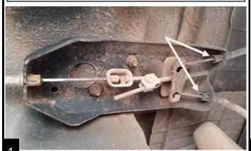
Raise the vehicle off the ground and support with jack stands. Remove brake drums and unhook the hard brake lines from the wheel cylinder using a 3/8" line wrench.
