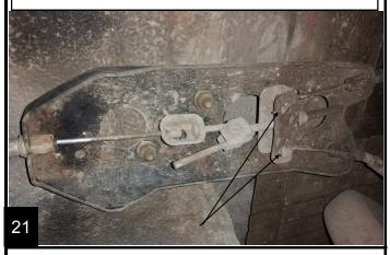
Adjust the parking/emergency brake until it holds the vehicle from moving while in gear.
