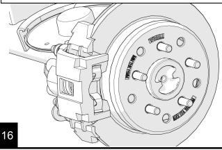
Install new brake hoses using new copper washers on the supplied banjo bolt. Install one copper washer onto the banjo bolt, slide the female end of the brake line onto the bolt, install another copper washer and install onto the caliper.
