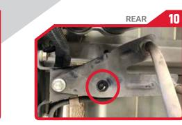
Loosen the remaining bolt.
