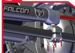
Torque stabilizer tie rod clam shell mount bolts to 15 ft. lbs. Reverify clearance and fitment.
