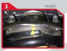
Before removing the strut assemblies mark the coil spring, spring isolator and strut tower to ensure the spring is reinstalled correctly. The spring must be reinstalled in the same orientation that it was removed.
