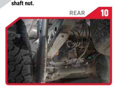
· Apply anti-seize to the shaft threads.
