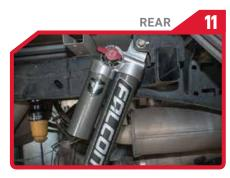
· Orient the passenger side reservoir to the rear with the roost guard facing to the
