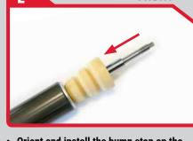
· Orient and install the bump stop on the shock shaft as shown.
