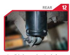
· Install the lower eyelet using the factory hardware and torque to 66 ft. lbs.
