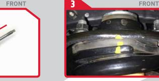
Before removing the strut assemblies mark the coil spring, spring isolator and strut tower to ensure the spring is reinstalled correctly.
