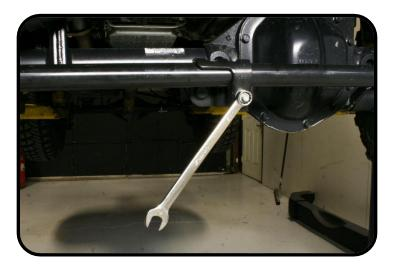
13. For the 2010-Current JK Wranglers: Using the factory hardware, install your new steering stabilizer with the dust shield to the axle side mount and the shock body to the tie rod mount. With an 18mm wrench tighten both ends and torque to 50 ft-lbs.
