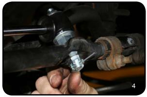
4. Insert new sleeve bushings into the newsteering stabilizer shock, make sure you use ones that fit your factory hardware. If tight, tap them in with a hammer. (Photo #5,6,)
