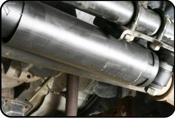
10. For the 2007-2009 JK Wranglers: Once the clearance is verified, tighten the U-bolt nuts to 35 ft\*lbs. Cycle the steering one more time to double check the clearance.
