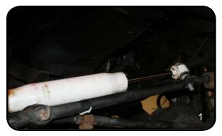
2. Install the new mounting pin into the steering stabilizer using the new nut and washers supplied and torque to 35 ft-lbs. (photo #2)
