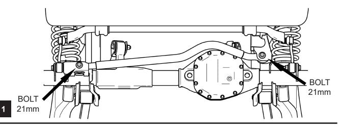
ADJUST THE NEW TRACK BAR TO THE APPROXIMATE LENGTH NEEDED TO CENTER THE AXLE UNDER THE JEEP
