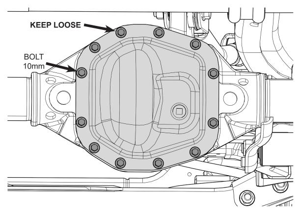
REMOVE AND DISCARD THE FACTORY DIFFERENTIAL COVER SEAL. THE FACTORY SEAL CANNOT BE USED WITH THE TERAFLEX COVER.
