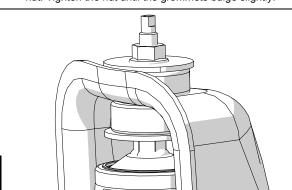
Reinstall the bolt and nut, torque to 56 ft-lbs.
