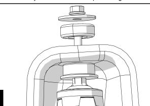
Remove the lower shock nut and bolt with an 18mm.
