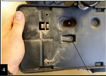
Disconnect the harness by pressing on the tabs and pulling the connection apart.
