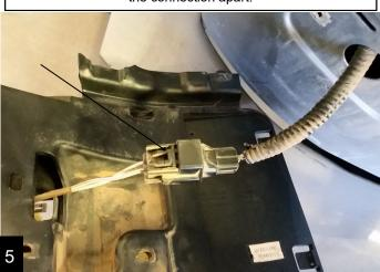
Tuck the harness back into the body and clean the recessed area thoroughly with soapy water.
