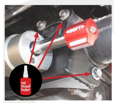
When installing the Falcon axle bracket, use the factory bolts and the provided **RED THREAD LOCKER**.
