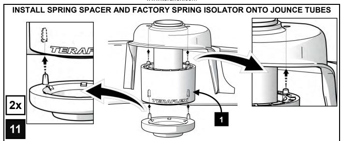
REINSTALL THE SPRINGS WITH LOWER BUMPSTOP SPACER INSIDE
