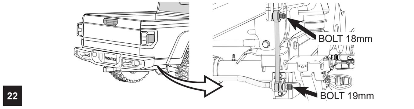
**TEMPORARILY REMOVE BRAKE LINE BRACKETS FROM BOTH SIDES OF THE FRAME**
