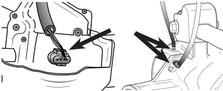
**RECONNECT PLASTIC RETAINERS FROM WIRING OR HOSES AS NEEDED.**
