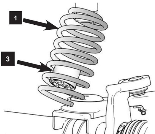
**INSTALL THE BUMPSTOP ONTO THE AXLE AND FULLY SEAT THE SPRINGS INTO THE LOWER SPRING PERCH**
