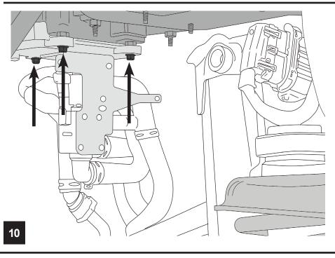
**REINSTALL TRAY TO VEHICLE WITH THE ORIGINAL 3 BOLTS** (10mm).
