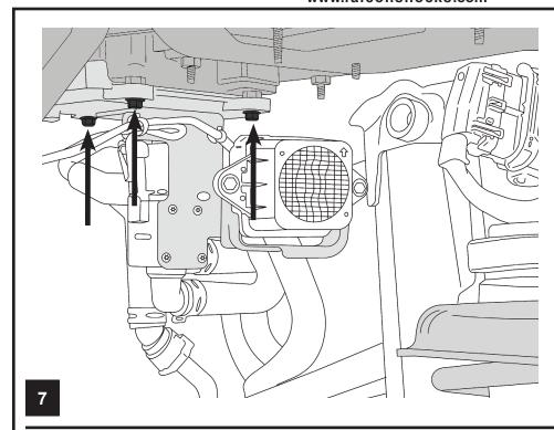
UNDO 3 BOLTS (10mm) SECURING TOP TRAY.
