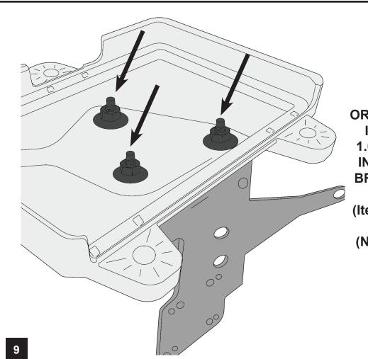
**USING THE 3 ORIGINAL NUTS AND INCLUDED (M6 x** 1.0 x 16mm) BOLTS **INSTALL THE NEW BRACKET TO TRAY.**
