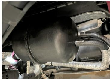
Align the Vacuum Canister with the new hole, insert bolts and tighten.
