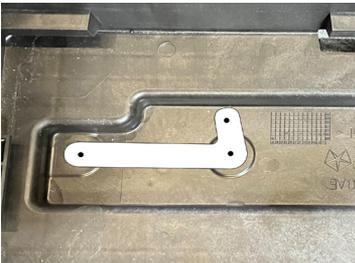
Place template as shown. Mark the new hole with a marker, then carefully drill with 1/4 inch drill bit.
