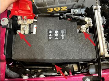
Using a 10mm wrench or socket, remove the negative battery terminal first, then the positive.
