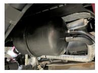
Align the Vacuum Canister with the new hole, insert bolts and tighten.
