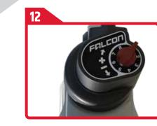
Adjust the 8-position knob to the desired firm setting. The shock adjusts from Soft to this setting when the in-cab switch is
