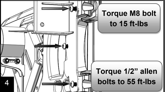
Install two 1/2"x3" bolts(4) and washers(3) through the outer most holes, from left to right. Then Install another washer(3) and a threaded spacer(2) onto the bolts. Finger tighten top bolt. Torque bottom bolt(13/16" wrench & 3/4" socket).
