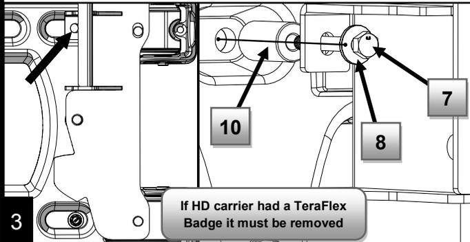
Install the 1/2" allen bolts(6) in the remaining holes using anti-seize to prevent thread corrosion. Note if upper 1/2" allen bolt does not line up with carrier, loosen upper left M8 bolt (as in step 2). Shift mount to line up holes and start 1/2" allen bolt. Retighten upper left M8 bolt.
