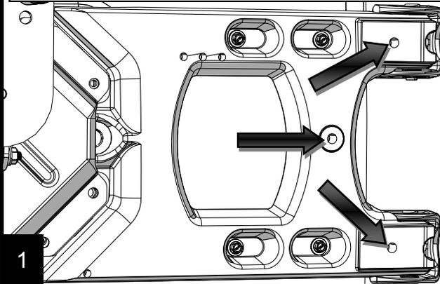
Using a 12mm socket remove the upper right M8 bolt that fastens the HD Hinged Carrier to the tailgate and loosen the other M8 bolt that is just to the left it. Note: These two bolts use the same floating captured nut plate inside the tailgate. By loosening the left bolt the plate will allow for better fitment.
