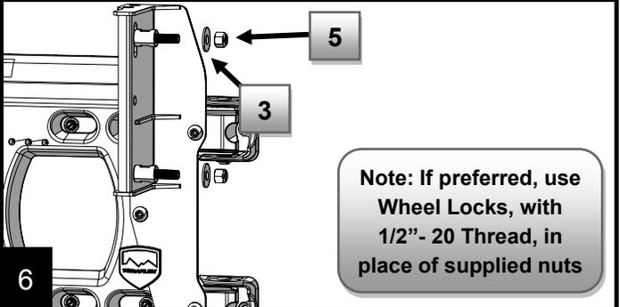
For the RotopaX Mount(1), that is purchased separately, install two 1/2 x 1.75" carriage bolts(5) through the mounts square holes and the Hi-Lift Jack. Fasten bolts with a washer (3) and nut(2). The RotopaX will be installed onto the four outer bolt holes.
