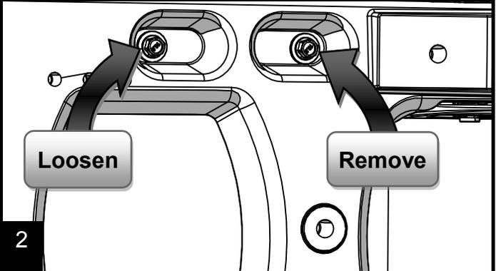
Position the mount and start the M8 bolt(7) and washer(8) into the mounts upper left hole, spacer(10) will go between the mount and carrier, leave bolt loose. Note: If there is a problems starting the M8 bolt, test fit spacer and bolt, without mount, to move nut into position. Next tighten the left bolt to keep plate in position, then remove spacer and M8 bolt, install as before.
