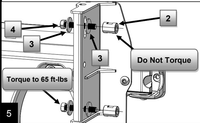
Have Hi-Lift Jack completely collapsed before installing. Push Hi-Lift Jack onto the bolts, adjust the top bolts position in slotted hole to best line up holes in the jack. Start 1/2" washers(3) and nuts(5) onto the 1/2" bolts(4), do not tighten nuts. With the top bolt lined up with the Hi-Lift Jack holes torque the top bolt to spacer (65 ft-lbs). Tighten both 1/2" nuts(5), securing the jack, then carefully check that the base of the jack will clear the body when the tailgate is fully open.
